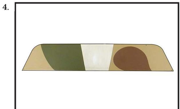
Slide the stabilizer partially into the fuselage so the wood at the center is exposed. Mix 1/2 ounce (15ml) of 30-minute epoxy. Use an epoxy brush to apply the epoxy to the exposed wood on the top of the stabilizer.
