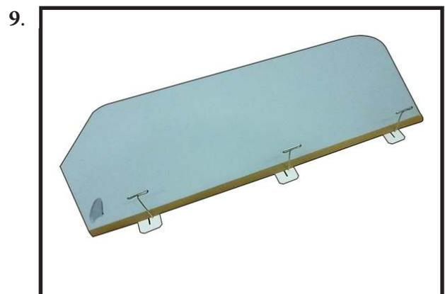
Fit the elevator into position on the stabilizer. Guide the joiner wire and hinges into position.
