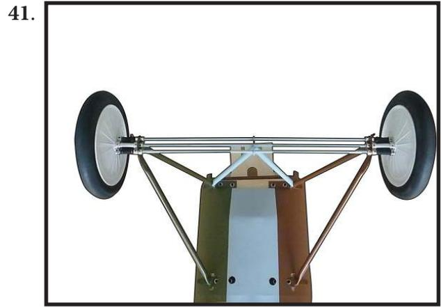
**INSTALLING THE STOPPER ASSEMBLY**
