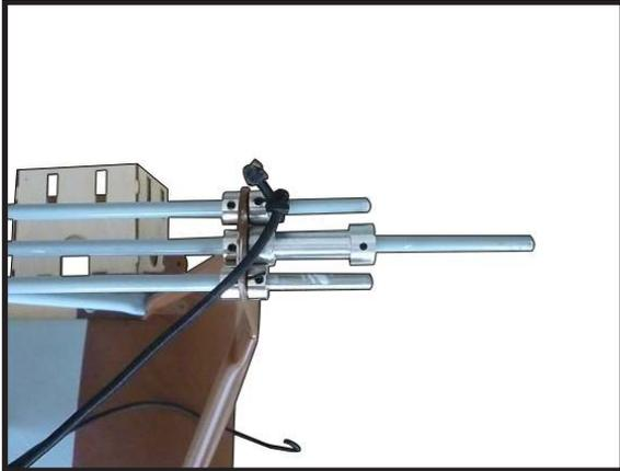
Wrap the shock cord under the shock cord collar on the main axle and under the forward axle support.
