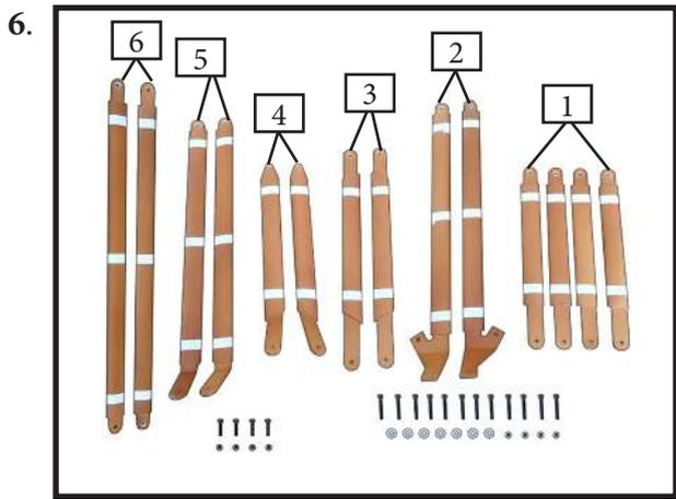
Get the middle number 1 strut and install it on the fuselage.
