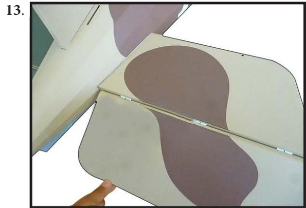
Flex the elevator slightly, making sure to keep the gap between the elevator and stabilizer as narrow as possible. Saturate each of the hinges using thin CA. Apply CA to the top of the hinges.
