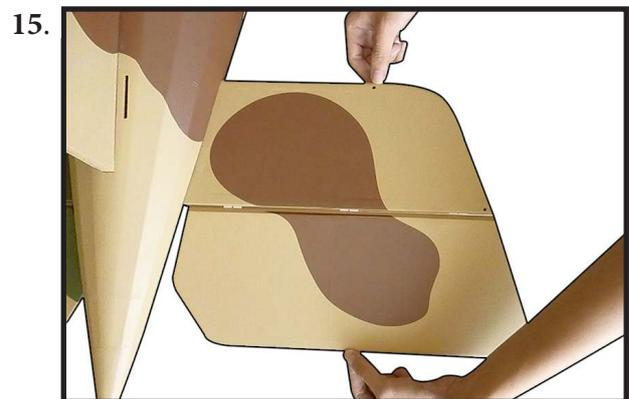
Flex the control surface through its range of motion a few 28. times to break-in the hinges. This will reduce the initial load on the servo when the surface is first actuated.
