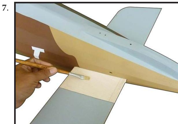
Once the alignment of the stabilizer has been verified, use a paper towel and isopropyl alcohol to remove any excess epoxy from the fuselage and stabilizer. Allow the epoxy to fully cure before proceeding.
