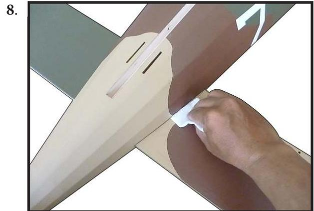
Use a pin vise and 1/16-inch (1.5mm) drill bit to drill a hole in the center of each hinge slot to allow the CA to wick into the hinge. Drill holes in both the elevators and stabilizer surfaces at this time. Place a T-pin in the center of each hinge along side the slot in the hinge. This will help center the hinge when it is placed in the elevators. Slide the hinges into position with the T-pin resting against the edge of the control surface.
