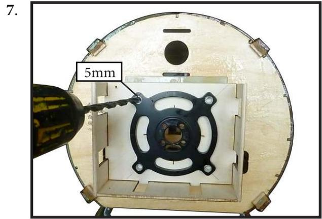
Then, use 5mm drill bit to enlarge the holes on the electric motor box.
