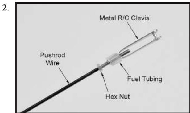
Locate items necessary to install rudder pushrod.
