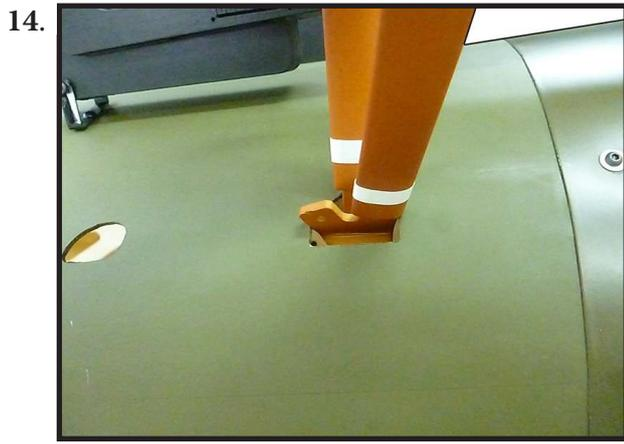
Get the middle number 3 strut and install it on the fuselage.
