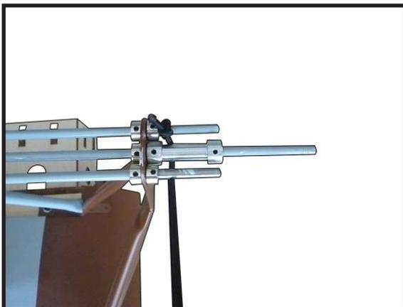
Loop the cord over the forward axle support, under the shock cord collar, then over the rear axle support.
