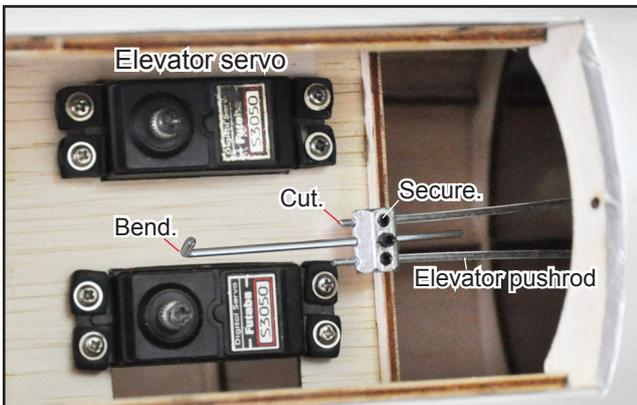
□ 1) Using pliers, carefully make a 90 degree bend down at the mark made. Cut off the excess wire, leaving about 6mm beyond the blend.
