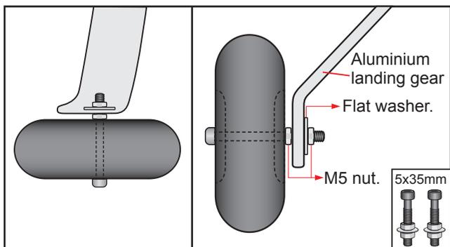
□ **3)** A drop of C/A glue on the wheel collar screws will help keep them from coming loose during operation.
