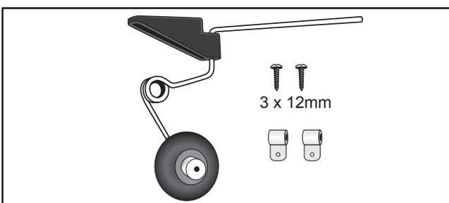
□ 3) Secure the tail wheel bracket in place using three 3mm x 12mm wood screws. Be careful not to overtighten the screws.
