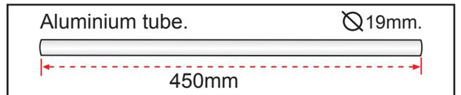
\*\*\* Test fit the aluminium tube dihedral brace into each wing haft. The brace should slide in easily. If not, use 220 grit sand around the edges and ends of the brace until it fits properly.
