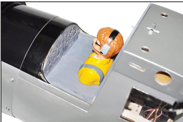
Position the canopy so the rear frame on the canopy is aligned with the rear edge of the cockpit opening. Use canopy glue to secure the canopy to the canopy hatch. Use low-tack tape to hold the canopy in position until the glue fully cures. Wrap the tape completely around the canopy hatch, as the tape does not stick well to the covering. We used balsa sticks to hold the lower edges of the canopy tightly against the canopy hatch.
