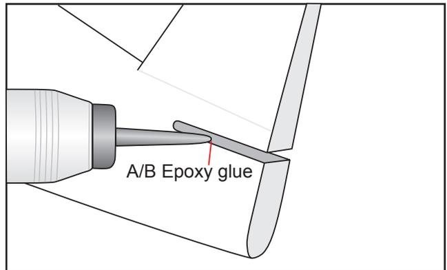
After the epoxy has fully cured, remove the masking tape or T-pins used to hold the stabilizer in place and carefully inspect the glue joints. Use more epoxy to fill in any gaps that may exist that were not filled previously and clean up the excess using a paper towel and rubbing alcohol.
