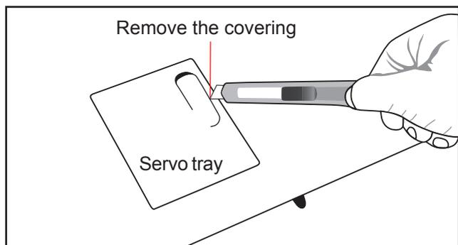
□ 3) Place the servo into the servo tray. Center the servo within the tray and drill 1.5mm pilot holes through the block of wood for each of the four mounting screws provided with the servo.
