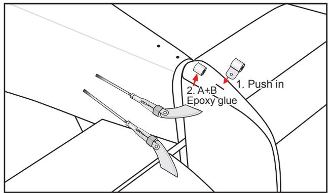
□ 2) Mark the locations of the two mounting screws. Remove the tail wheel bracket and drill 2mm pilot holes at the locations marked.
