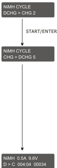
After selecting the correct battery type, use the INC or DEC button to select the “CYCLE” mode. The Cycle Mode gives you two cycling options: “DCHG>CHG” or “CHG>DCHG”. The “DCHG>CHG” option will first discharge the battery and then recharge the battery.
