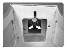
This step may require additional sanding of the fuselage fuel tank former.
