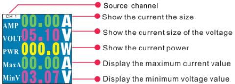
When the voltage less than the set value, current more than the set, will show a warning While the voltage or current will be highlighted.
