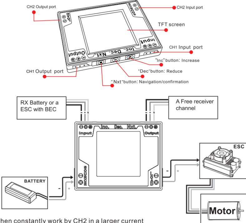
★ When constantly work by CH2 in a larger current circumstances, it may need to add a cooling device (shown below), or may cause the display does not work, even damage the display.
