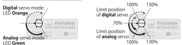
When a remote gain function is off, it becomes only analog servo mode. A trimmer becomes only for gain.
