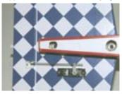
Tail servos are mounted in the flying surfaces - two bolts hold the tail on.
