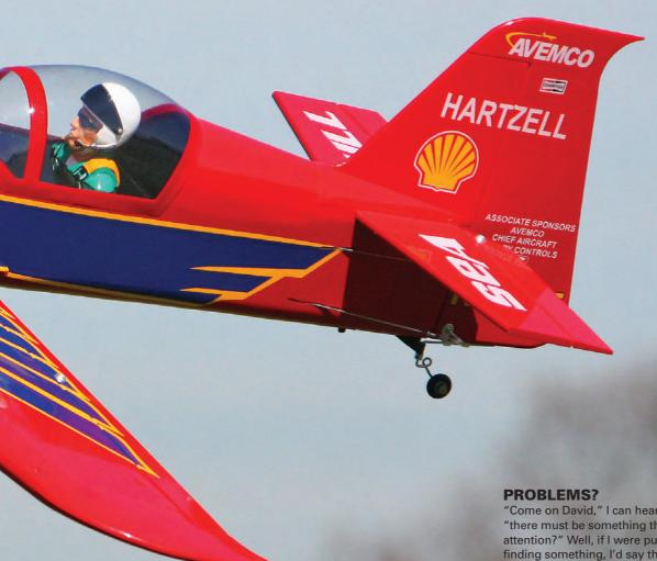
Seagull could have run shy of reproducing the Raven's distinctive wing tips and employed stick-on plastic mouldings instead, but it hasn't. To its credit, then, the all-wood, film-covered tips are top drawer. This quality level continues throughout the airframe, indeed particularly impressive is the moulded fibreglass cowl, which is
