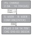
When you are willing to alter the parameter value in the program, press Enter key to make it blink, then change the value with INC/DEC key the value will be stored by pressing Enter key once then press Enter key for more than 2 seconds to start the process.
