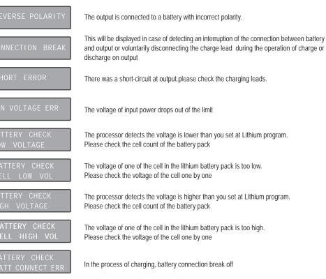
The voltage of input power drops out of the limit
