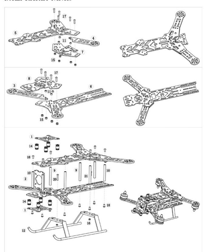
Note: You have two ways of assembling part ① as shown in the above diagram. Install motors as it is shown in the diagram on the right.
