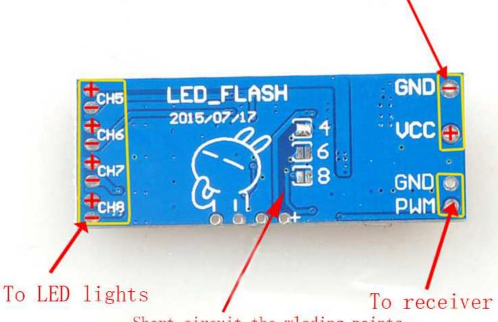
Short circuit the wleding points next to 4 for quadcopters, and 6 for hexacopters and so on.
