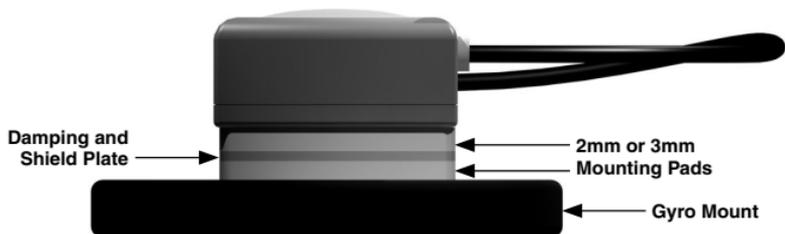
On smaller electric helicopters it is best to mount the gyro using one 2mm mounting pad. When mounting the gyro in a larger electric or .50 through .91 size nitro helicopter we recommend using two 3mm Mounting Pads and the Damping/Shield Plate.
