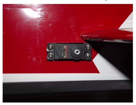
31. Electronically center the servo and install the longest servo arm from the Dubro servo arm kit. Locate the longest pushrod and 2 ball links and assemble the pushrod linkage as shown in the picture below. Remember to use Loctite on all nuts.
