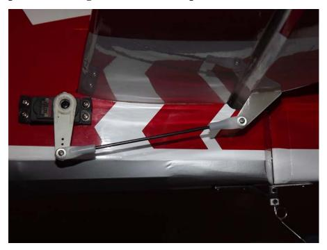
32. Using the same procedure as with the elevator, install the rudder servo on the right side of the fuse with the output shaft toward the rear of the aircraft. Locate the middle sized pushrod and 2 ball links and assemble the pushrod linkage as shown in the picture below. Remember to use Loctite on all nuts.
