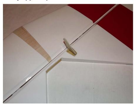
23. Slide the elevator onto the hinges in the stabilizer making sure the hinges are centered in the hinge gap and secure with thin CA.
