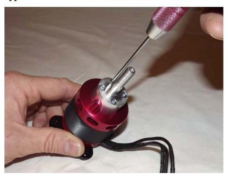
36. Mount the Torque motor using the supplied 4mm black socket head cap bolts and washers. The bolts are to be inserted into the blind nuts which are pre-installed in the motor mount plate. Be sure to put a drop of blue Loctite onto each bolt to prevent them from backing out. Also take time to add CA to all motor box joints!
