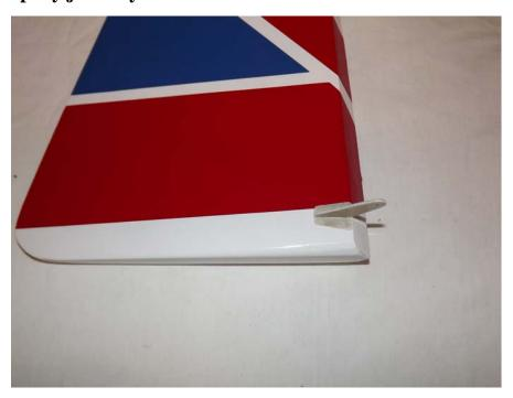
28. Slide the rudder onto the hinges in the vertical stab, making sure the hinges are centered between the rudder and stab. Also, make sure the rudder is flush with the top and bottom of the stab. Once satisfied, glue the hinges in place with thin CA making sure the rudder is fully deflected.
