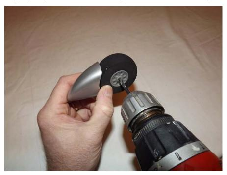
15. Insert the threaded portion of axel through the spat, then mount the axel and spat onto the landing gear by attaching the lock nut and washer onto the axle. Tighten the nut, making sure the wheel spat is positioned properly.
