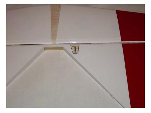
22. Scuff the portion of the control horn that will insert into the elevator as well as the bottom of the base plate with sandpaper. Secure the control horn to the elevator with epoxy just as you did with the aileron horns.
