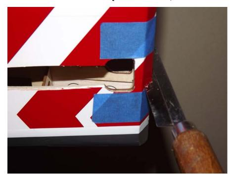
20. Locate the horizontal stabilizer/elevator assembly. Turn it upside down on your building table and remove the covering over the right slot on the bottom of the elevator where the elevator control horn will be installed. Using the same process as with the ailerons, insert the horn into the base plate and into the slot. Trace around the base plate with a fine tipped marker.
