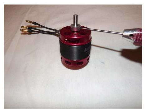
34. Next, secure the radial mount to the motor using the provided short Phillip's head machine screws. Again be sure to use a drop of blue Loctite on each screw.
