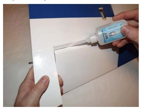
9. Before installing the aileron servo, take a minute and apply some CA to the servo tray and the anti-rotation pins.
