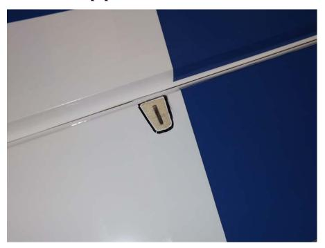
4. Use sandpaper to scuff the portion of the horn that will be inserted into the aileron as well as the bottom of the base plate.
