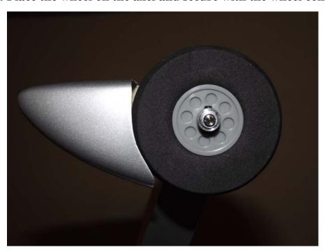
17. When satisfied with the position of the wheel pant, drill a 1/16<sup>th</sup> hole through the wheel spat at the location of the hole in the landing gear and secure with a wood screw. Repeat this process for the remaining wheel and spat.
