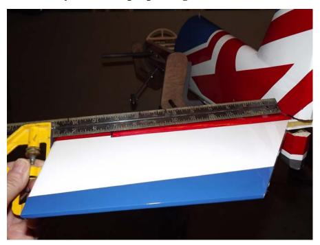
25. Once satisfied with the alignment, glue the horizontal stab in place by applying CA along the joint between the stab and fuse. Make sure to apply CA to the top and bottom of the stab, being careful not to get CA on the covering.
