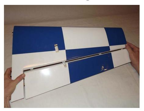
8. Making sure the aileron is properly aligned between the wing root and wing tip, hold the aileron fully deflected and apply a drop of thin CA to each hinge. Flip the wing over and repeat.
