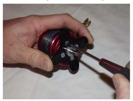
35. Secure the prop adapter using the 4 socket head cap bolts. Blue Loctite should be applied to each bolt.
