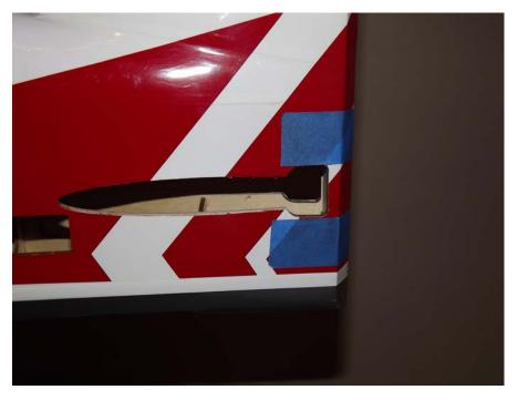
19. Use a razor saw to carefully make the cut, then sand smooth.
