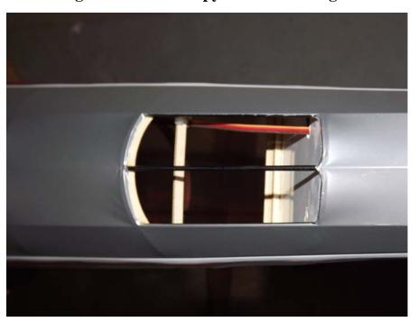
42. The wings are retained by inserting the 4MM nylon bolts through the holes in the fuselage just behind the wing tube and into the pre-installed blind nuts in the root rib of the wing. Be careful not to cross thread the bolts and inspect them periodically to insure thread integrity.
