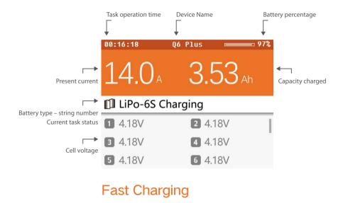
Rotating the shuttle key during operation can switch the displayed information in the lower half of the screen, which are cell voltage, cell internal resistance and working parameter. The cell voltage and internal resistance can only be displayed in the mode of balance charging (3 minutes).
