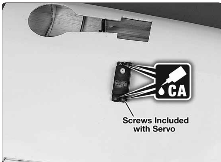
❑ 4. Install servo screws.
