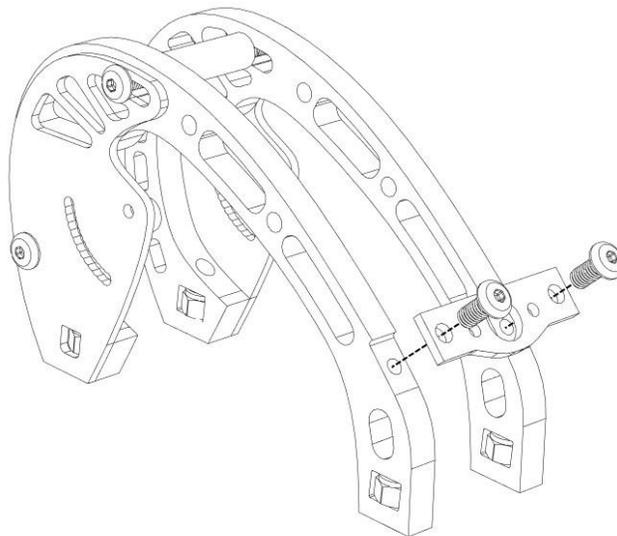
Step 5 – The top section is mounted with 2x M3x14mm bolts (back) and 2x M3x 12mm bolts (front). If you don't use the XT60 connector bracket, you can use 2x M3x12mm instead of M3x14mm.
