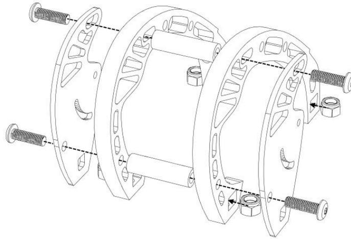
Step 4 – Put the small 2mm thick antenna plate on top of the backside of the aluminum brackets and secure it with 2x M3x6mm.
