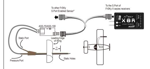
\*Install FrSky Smart Port Air Speed Sensor ASS-70/ASS-100 on any appropriate surface of the airframe that stays away from water, vibration, or fuel.
