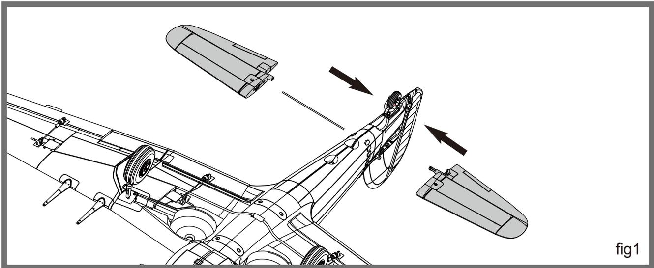
2. Secure the horizontal tail piece in place using the include screw: PA2.6\*10. Use caution to avoid over-tightening the screw.
