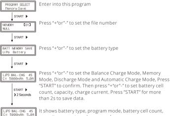
It shows battery type, program mode, battery cell count, capacity, current you have saved.
