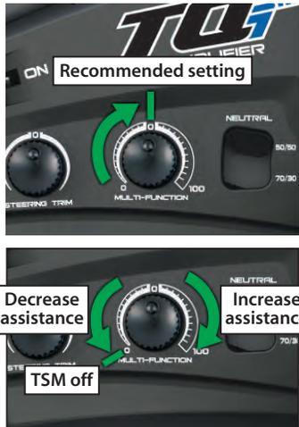
When driving on surfaces with some traction, decrease the TSM setting to allow the vehicle to feel more "loose" for power sliding, drifting, and so on. On surfaces with very little traction (loose dirt, smooth concrete, ice/snow), increase TSM to maximize acceleration and control.
