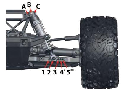
The suspension of your model has been set up for off-road performance (position 2 on the front suspension arms and position 3 on the rear suspension arms). If you plan on driving on hard surfaces, the following changes should be made:
