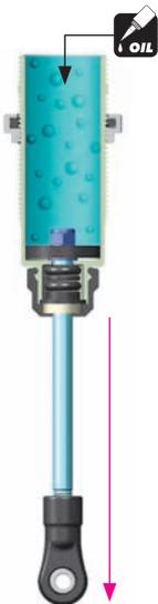
1 Extend the shock shaft completely. Fill the shock body with the shock oil. For the shocks use 1000cSt oil.
