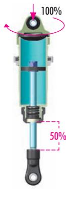
6 Keep the shock shaft pushed 50% into the shock body and tighten the shock cap completely. The rebound will be at approximately 50%.
