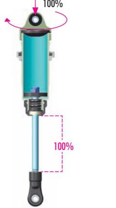
4 Gently place the shock cap assembly onto the filled shock body. Keep the shock shaft extended 100% from the shock body and tighten the shock cap completely. The rebound will be at approximately 100%.
