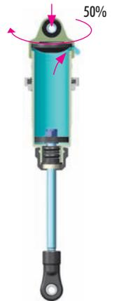
4 Gently place the shock cap assembly onto the filled shock body. Excess oil will spill from the shock.
