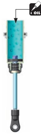
2 Fill the shock body with shock oil up to the top. Make sure to use same viscosity shock oil as is in the shock.
