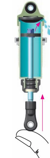
6 Gently push the shock shaft completely into the shock body. Excess oil will flow through the hole in the shock cap.
