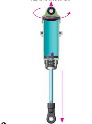
1 Extend the shock shaft completely and remove the shock cap.
