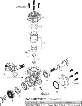
79871030 M2.6x10 Cylinder Head Retaining Screw (4pcs.)
