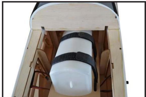
7) Slide the fuel tank into the fuselage. Guide the lines from the tank through the hole in the firewall.
