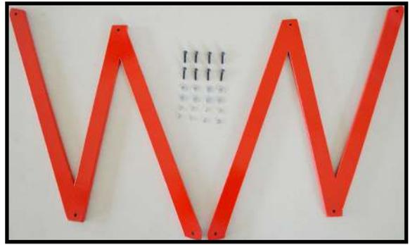
2) Attach the two wing struts to the top of lower wing panel using an M3x12mm machine screw and M3 washers.
