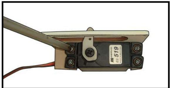
6) Apply 1-2 drops of thin C/A to each of the mounting tabs. Allow the C/A to cure without using accelerator.
