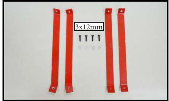
2) Place the cabane struts in position, noting their position as shown in the photo. Loosely install the four M3 x 12 socket head machine screws and M3 washers. Leave the hardware loose so the struts can be positioned while installing the upper wing center rib. Make sure to use threadlock on the screws so they won't vibrate loose.
