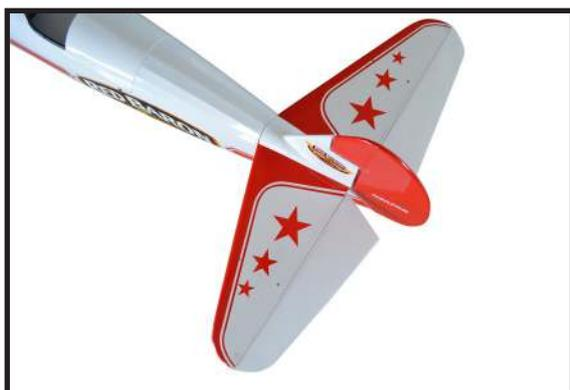
5) When you are sure that everything is aligned correctly, mix up a generous amount of Flash 30 Minute Epoxy. Apply epoxy to the bottom and top edges of the filler block. Set the stabilizer in place and realign. Double check all of your measurements once more before the epoxy cures. Hold the stabilizer in place with T-pins or masking tape and remove any excess epoxy using a paper towel and rubbing alcohol. Allow the epoxy to fully cure before proceeding.
