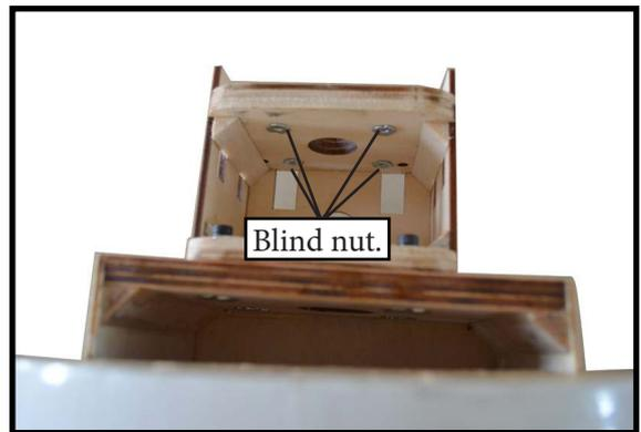
4) Attach the motor to the front of the electric motor box using four 4mm blind nut, four M4x20mm hex head bolts to secure the motor. Please see picture shown.
