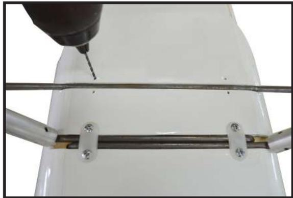
Thread a mounting screw into each of the holes to cut threads in the surrounding wood. Apply a small amount of thin CA to harden the threads made by the screws. Position the landing gear so it rakes forward. Use the screws and landing gear straps to secure the landing gear to the bottom of the fuselage.
