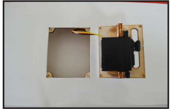
8) Set the aileron hatch in place and use a Phillips screw driver to install it with four wood screws.
