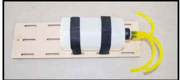
**!** You should mark which tube is the vent and which is the fuel pickup when you attach fuel tubing to the tubes in the stopper. Once the tank is installed inside the fuselage, it may be difficult to determine which is which.
