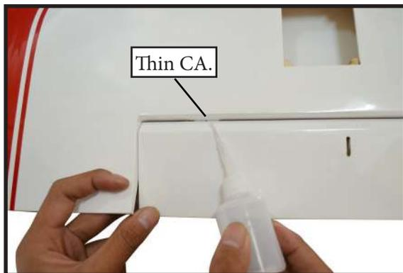
5) Turn the wing panel over and deflect the aileron in the opposite direction from the opposite side. Apply thin C/A glue to each hinge, making sure that the C/A penetrates into both the aileron and wing panel.
