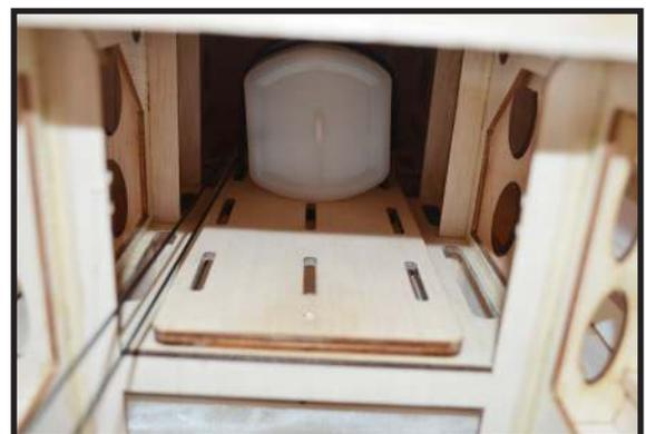
8) Use balsa block to hold in place the fuel tank with C/A glue to secure the fuel tank inside the fuselage.
