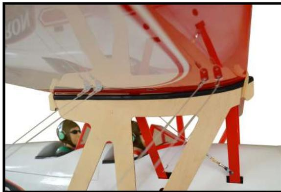
2) Use a 2.5mm hex wrench to remove the screws that attach the panels to the fuselage and center section. Slide the panels from the tubes and disconnect the servo lead for the aileron servo.
