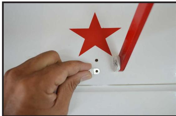
*At this time, exact position of the end is set, please Use a 2.5mm hex wrench to slowly tighten the hardware securing the cabane struts in position on the fuselage. Again, make sure to use threadlock on all the fasteners to prevent them from vibrating loose.*
