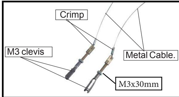
2) Attach the clevis to the brass tab next to the rear interplane strut on the upper-lower wing. Slide a copper crimp on the cable. Pass the cable through the brass tab on the upper wing, the back through the copper crimp.
