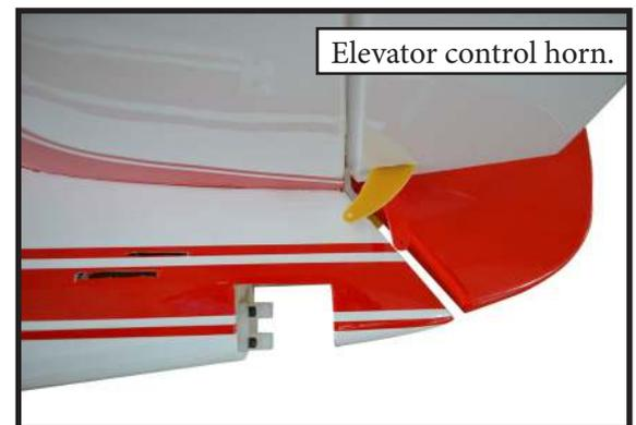
3) Thread one clevis and M2 lock nut on to each elevator control rod. Thread the horns on until they are flush with the ends of the control rods.
