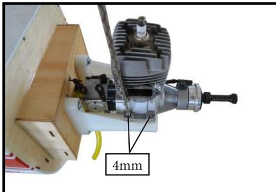
3) Use a drill to drill the four holes in the engine mount rails.
