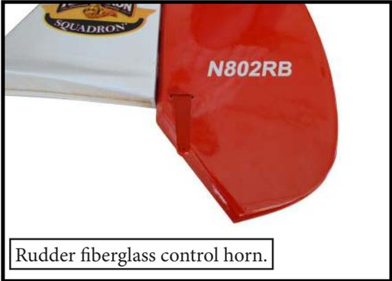
Rudder fiberglass control horn.
