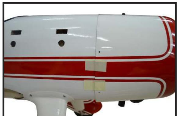
2) Use a drill and drill bit to drill the holes for the cowl mounting screws. Make sure the cowl position is correct before drilling each hole.
