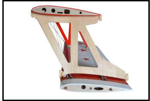
*Using the transport frames allow the removal of the wings without the need to remove the aileron linkage and the inter-plane strut between the top and bottom wings.*
