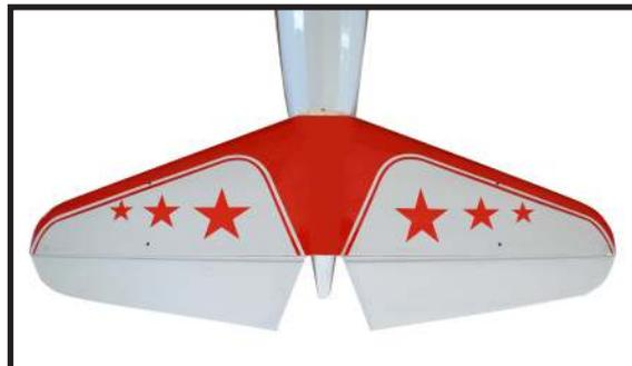
4) With the stabilizer held firmly in place, use a pen and draw lines onto the stabilizer where it and the fuselage sides meet. Do this on both the right and left sides and top and bottom of the stabilizer.
