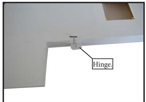
3) Slide the wing panel on the aileron until there is only a slight gap. The hinge is now centered on the wing panel and aileron. Remove the T-pins and snug the aileron against the wing panel. A gap of 1/64" or less should be maintained between the wing panel and aileron.
