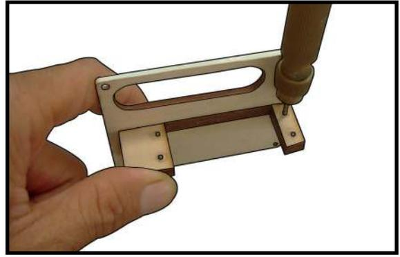
3) Apply 2-3 drops of thin C/A to each of the mounting holes. Allow the C/A to cure without using accelerator.
