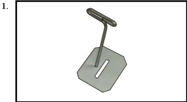
2) Remove each hinge from the wing panel and aileron and place a T-pin in the center of each hinge. Slide each hinge into the wing panel until the T-pin is snug against the wing panel. This will help ensure an equal amount of hinge is on either side of the hinge line when the aileron is mounted to the aileron.
