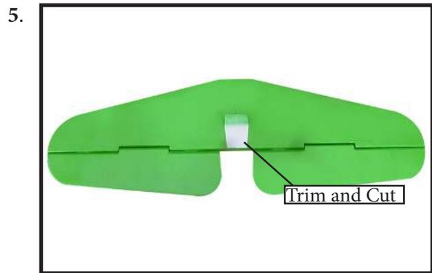
**⚠ When cutting through the covering to remove it, cut with only enough pressure to only cut through the covering itself. Cutting into the balsa structure may weaken it.**
