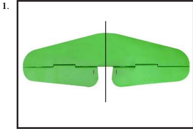
2) Using a modeling knife, carefully remove the covering at mounting slot of horizontal stabilizer ( both side of fuselage).
