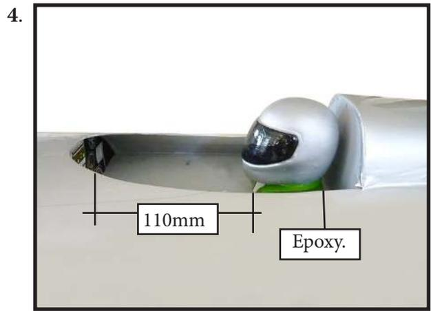
4) Epoxy canopy onto the fuselage. Trace around the canopy and onto the fuselage using a epoxy.
