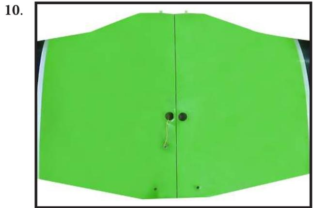
6) Apply 1-2 drops of thin C/A to each of the mounting tabs. Allow the C/A to cure without using accelerator.
