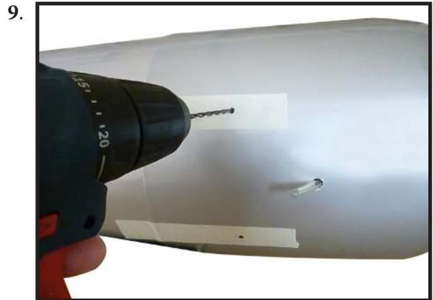
3) With the muffler, needle valve, and spark/ glow plug removed from the engine, slide the cowl in place over the engine. Temporarily install the propeller and spinner in order to find the exact location of the cowl. When satisfied with the cowl placement, secure the cowl to the fuselage using masking tape.
