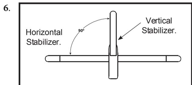
4) Slide the vertical stabilizer back in place. Using a triangle, check to ensure that the vertical stabilizer is aligned 90° to the horizontal stabilizer.
