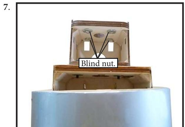
5) Attach the motor to the front of the electric motor box using four 4mm blind nut, four M4x20mm hex head bolts to secure the motor. Please see picture shown.
