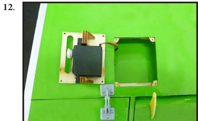
8) Set the aileron hatch in place and use a Phillips screw driver to install it with four wood screws.
