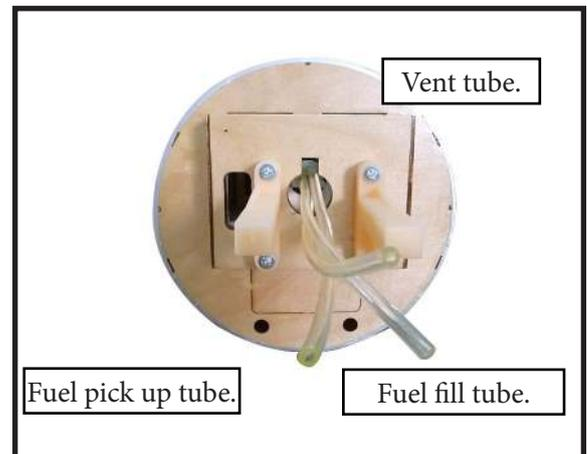
8) Connect the lines from the tank to the engine and muffler. The vent line will connect to the muffler and the line from the clunk to the carburetor.
