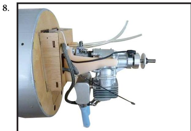
8) Reinstall the servo horn by sliding the connector over the pushrod wire. Center the throttle stick and trim and install the servo horn perpendicular to the servo center line.
