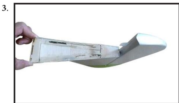
2) Slide the vertical stabilizer into the slot in the top of the fuselage. The rear edge of the stabilizer should be flush with the rear edge of the fuselage and the lower rudder hinge should engage the precut hinge slot in the lower fuselage. The bottom edge of the stabilizer should also be firmly pushed against the top of the horizontal stabilizer.
