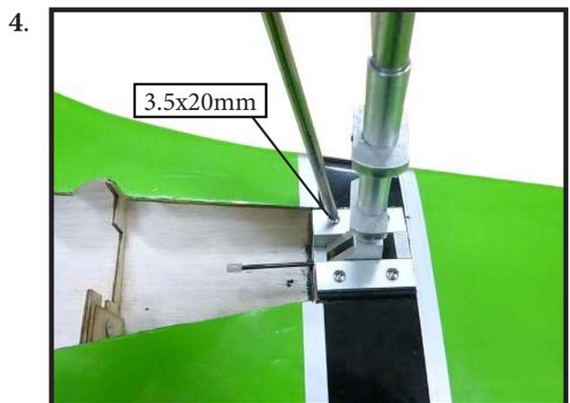
2) Install servo for Retractable landing gear.
