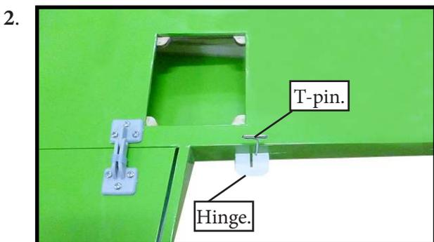
3) Slide the wing panel on the aileron until there is only a slight gap. The hinge is now centered on the wing panel and aileron. Remove the T-pins and snug the aileron against the wing panel. A gap of 1/64" or less should be maintained between the wing panel and aileron.
