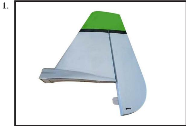
1) Using a modeling knife, remove the covering from over the precut hinge slot cut into the lower rear portion of the fuselage. This slot accepts the lower rudder hinge.
