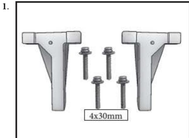
2) Use four 4x30mm head bolts and four 4mm washers to attach the engine mount rails to the firewall. Tighten the screws. Make sure to use threadlock on the screws to help prevent them from vibrating loose.
