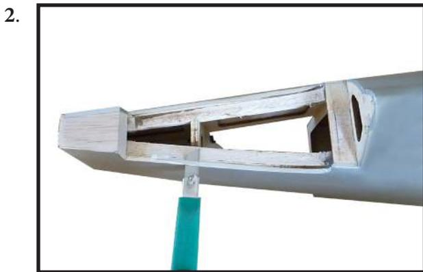
3) Slide the stabilizer into place in the precut slot in the rear of the fuselage. The stabilizer should be pushed firmly against the front of the slot.
