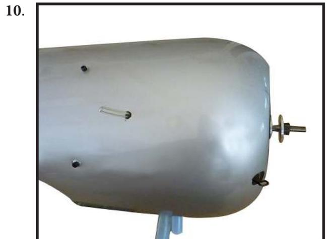
4) Install the muffler and muffler extension onto the engine and make the cutout in the cowl for muffler clearance. Connect the fuel and pressure lines to the carburetor, muffler and fuel filler valve. Secure the cowl to fuselage using the M3x10mm socket head screws. Putting a small length of silicon fuel tube under the head of the screw helps with vibration.
