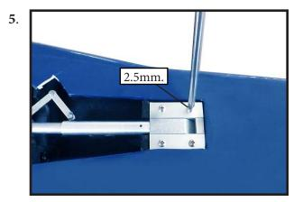
Install servo for Retractable landing gear.
