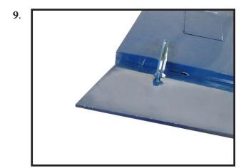
Once adjusted, make sure all clevis retainers are in position. Apply a drop of threadlock near the clevis, then tighten the nut against the clevis to keep the linkage from changing length inside the wing.
