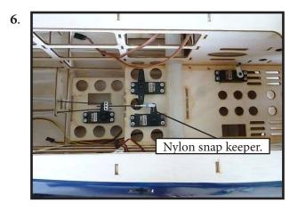
**RUDDER PUSHROD INSTALLATION**
