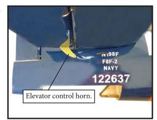
Thread one clevis and M2 lock nut on to each elevator control rod. Thread the horns on until they are flush with the ends of the control rods.
