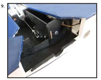
Slide the wheel on the axle, then secure it using the wheel collar.
