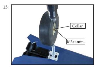
Secure the landing gear doors to the landing gear struts.
