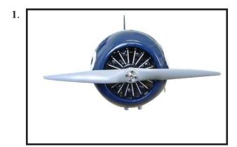
The propeller should not touch any part of the spinner cone. If it does, use a sharp modeling knife and carefully trim away the spinner cone where the propeller comes in contact with it.
