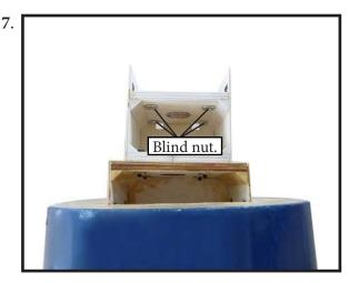
5) Attach the motor to the front of the electric motor box using four 4mm blind nut, four M4x20mm hex head bolts to secure the motor. Please see picture shown.
