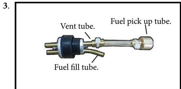
Carefully bend the second nylon tube up at a 45° angle. This tube is the vent tube.
