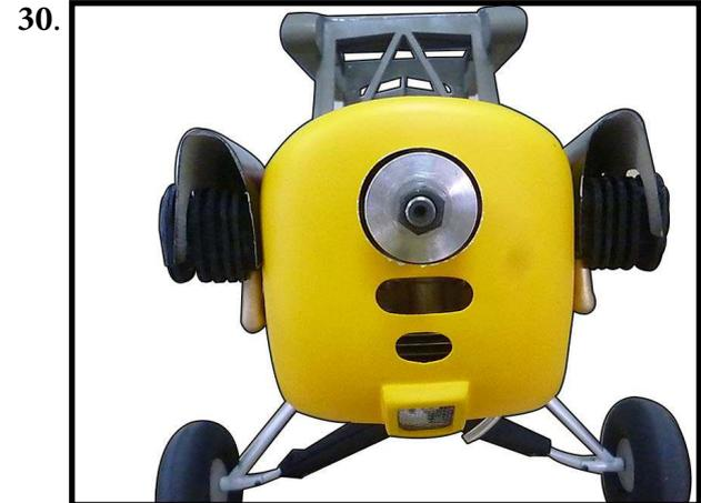
*Because of the size of the cowling, it may be necessary to use a needle valve extension for the high speed needle valve. Make this out of sufficient length 1.5mm wire and install it into the end of the needle valve. Secure the wire in place by tightening the set screw in the side of the needle valve.*
