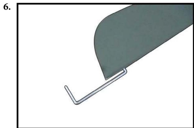
The elevator joiner wire must be flush with the leading edge of the elevator as shown.
