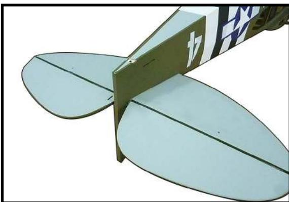
Use a small strip of the clear packaging material and slide it between the joiner wire and stabilizer. Make sure the packing material is cut so it does not obstruct the hinge slot. Use a small piece of low-tack tape to hold the packing material in position.
