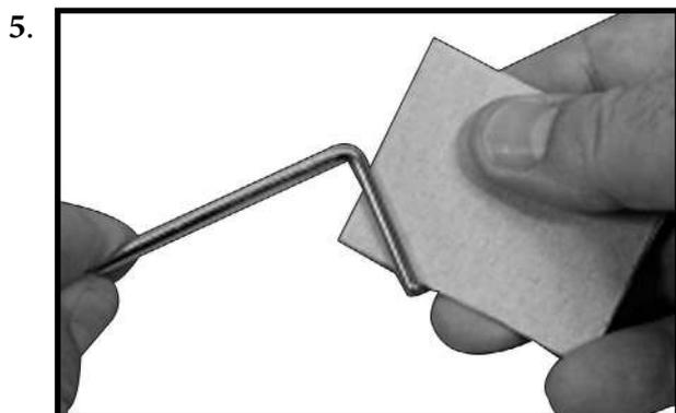
Fit the joiner wire into the elevator halves.
