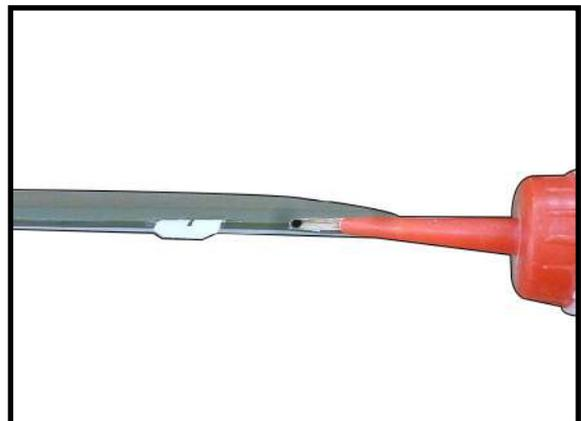
Fit the elevators back into position. Remove the T-pins and slide the elevators tightly against the stabilizer. Use a paper towel and isopropyl alcohol to remove any excess epoxy before it begins to cure.
