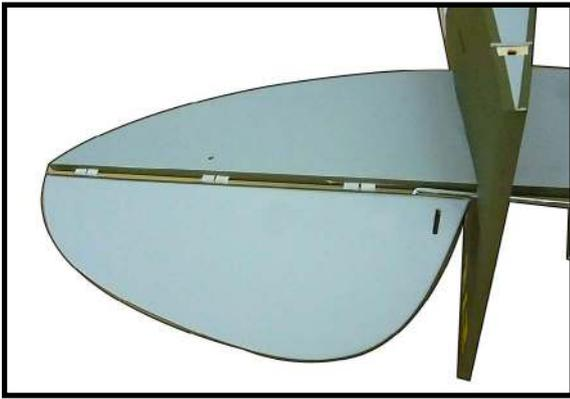
Fit the elevator so the leading edge fits tightly against the trailing edge of the stabilizer.
