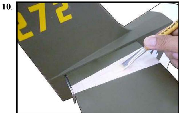
Carefully turn the model over and apply epoxy to the exposed wood on the bottom of the stabilizer. Slide the stabilizer back into position.
