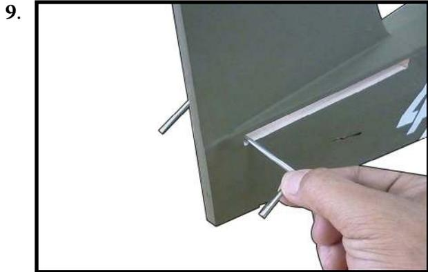
Slide the stabilizer partially into the fuselage so the wood at the center is exposed. Mix 1/2 ounce (15ml) of 30-minute epoxy. Use an epoxy brush to apply the epoxy to the exposed wood on the top of the stabilizer.
