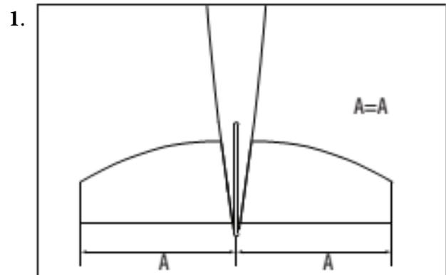
Measure from the tip of the stabilizer to the wing. Position the stabilizer so both measurements are equal. (Cowling has not been installed at this time.)
