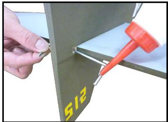
Use a toothpick to apply epoxy to the stabilizer where it contacts the joiner wire.
