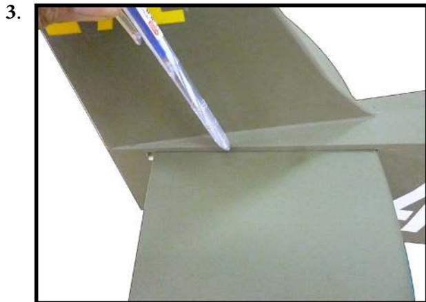
Use a ruler and carefully cut the covering 1/8 inch (3mm) inside the line drawn on the stabilizer to remove the covering from the center of the stabilizer. Remove the top and bottom covering. Use care not to cut into the underlying wood, weakening the stabilizer.
