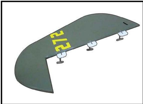
Check the fit of the rudder to the fuselage. Make sure the tail wheel wire fits into the rudder, and that the notch fits over the tail wheel bushing. There should be no gap between the fin and rudder.
