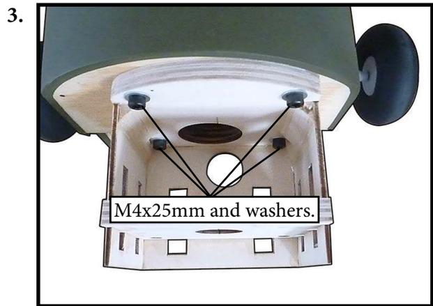
Attach the motor to the front of the electric motor box using four 4mm blind nut, four M4x25mm hex head bolts to secure the motor. Please see picture shown.
