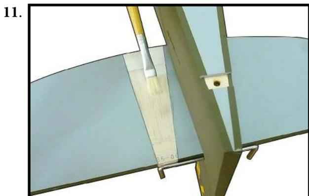
Once the alignment of the stabilizer has been verified, use a paper towel and isopropyl alcohol to remove any excess epoxy from the fuselage and stabilizer. Allow the epoxy to fully cure before proceeding.
