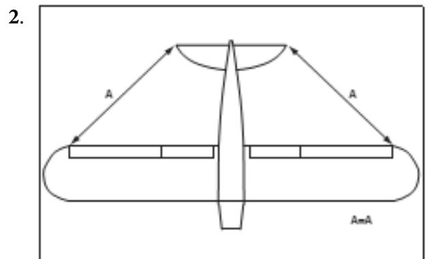
Check all alignments. Mark the outline of the fuselage on the top and bottom of the stabilizer.
