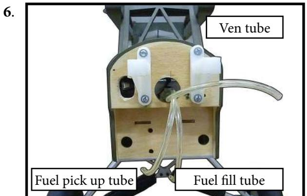
Connect the lines from the tank to the engine and muffler. The vent line will connect to the muffler and the line from the clunk to the carburetor.
