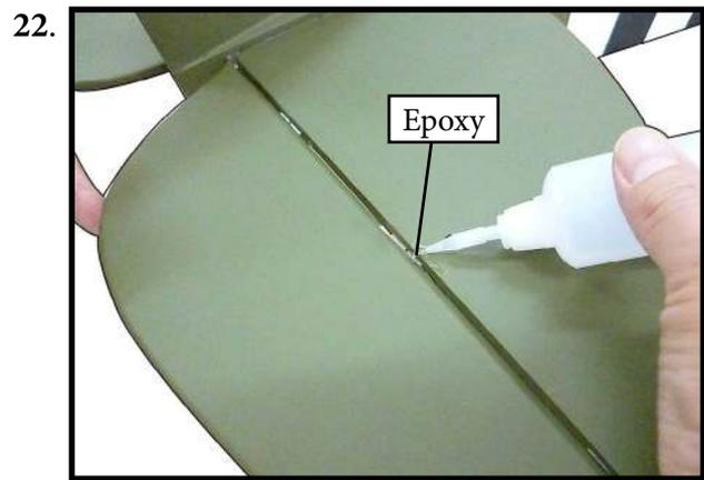
Flex the elevator slightly, making sure to keep the gap between the elevator and stabilizer as narrow as possible. Saturate each of the hinges using thin CA. Apply CA to the bottom of the hinges. Allow the CA to cure before proceeding.
