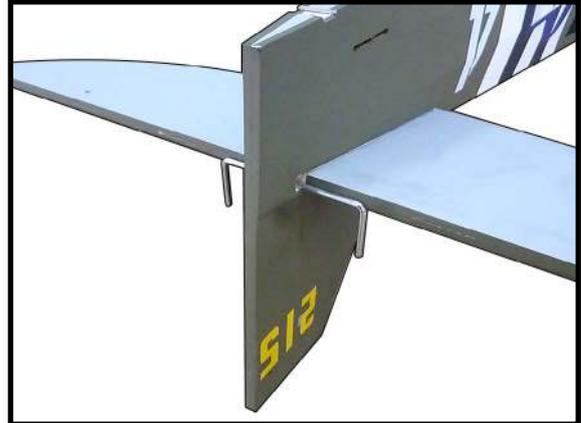
Mix a small amount of 15-minute epoxy. Use a toothpick to apply epoxy to the joiner wire.
