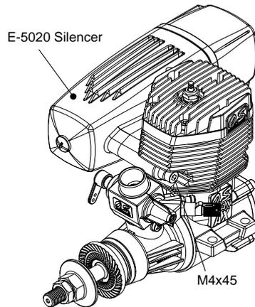
■ **In case of installing the silencer with the extension adaptor to the engine**
