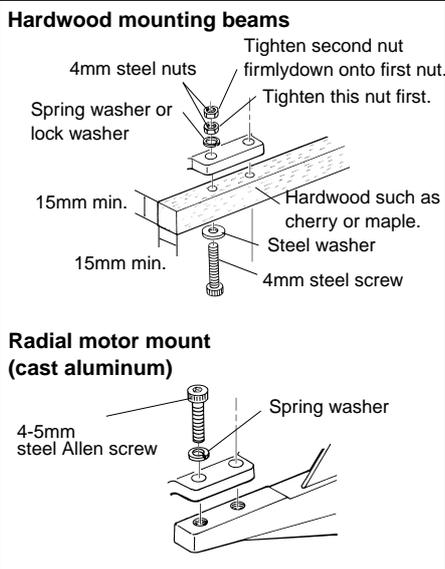
Make sure that these mounting beams are accurately aligned and firmly integrated with the airframe, reinforcing the adjacent structure to absorb vibration. Use 4mm or larger steel screws, preferably Allen type hexagon socket head cap screws, with washers and locknuts, for bolting the engine to the bearers.
