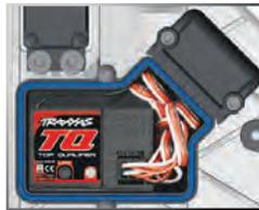
**Note: For best performance, it is recommended that the receiver be installed in the original orientation as shown.**
