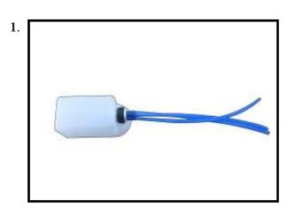
You should mark which tube is the vent and which is the fuel pickup when you attach fuel tubing to the tubes in the stopper. Once the tank is installed inside the fuselage, it may be difficult to determine which is which.
