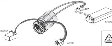
Insert the throttle cable of the ESC into the throttle channel of receiver. Because the red line of throttle cable output 6V/7.4V voltage to receiver and steering servo, do not supply power to receiver, otherwise the ESC may be maged. If need to supply power, pick out the red line among throttle cable, wrap it and suspend.
