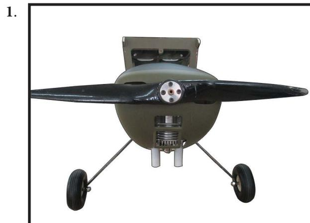
⚠ The propeller should not touch any part of the spinner cone. If it does, carefully trim spinner cone opening until propeller no longer comes in contact with it.
