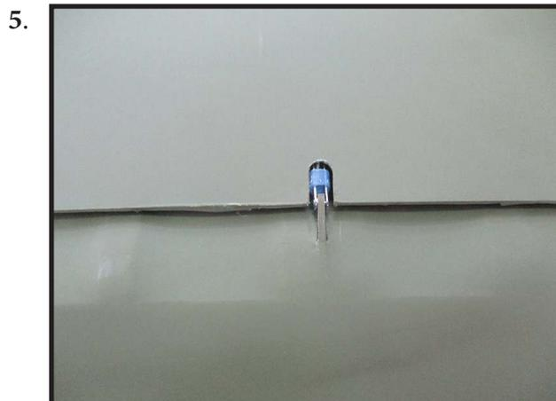
Attach the clevis to the flap servo arm.
