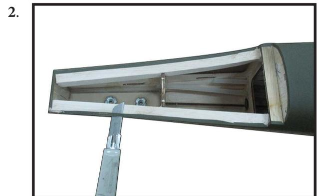
Slide the stabilizer into place in the precut slot in the rear of the fuselage. The stabilizer should be pushed firmly against the front of the slot.
