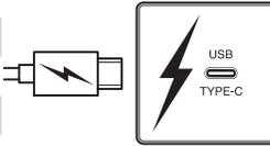
1. Plug the USB-C cable into a USB-C power source. The red LED will turn on, indicating that power is connected.
