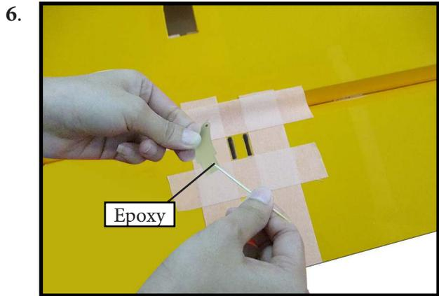
Before the epoxy fully cures, remove the tape from around the control horn. This will allow the epoxy to flow around the control horn, creating a small fillet between the control horn and surface for a finished look and secure bond.
