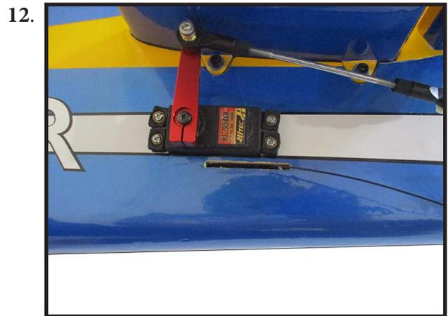
Thread cable through brass swage tube.
