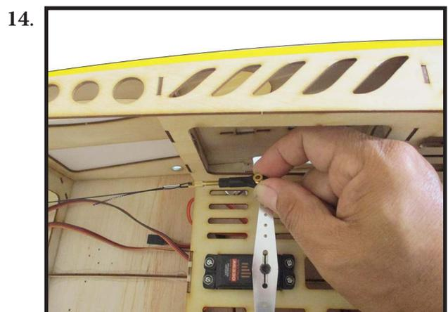
Crimp the brass swage tube with a crimping tool or pliers.
