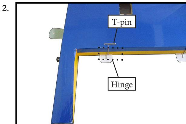
Slide the wing panel on the flap until there is only a slight gap. The hinge is now centered on the wing panel and flap. Remove the Tpins and snug the flap against the wing panel. A gap of 1/64" or less should be maintained between the wing panel and flap.
