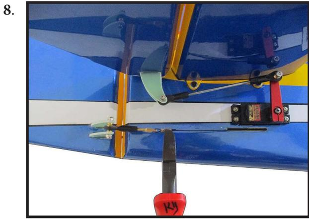
Cut off excess cable as shown.
