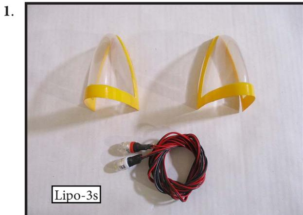
The green light for right wing tip, and the red light for left wing tip. They are designed to operate on voltages 12 volts. Connect four lights into switch circuit so that optional the different flashes mode.
