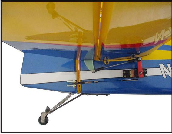
**INSTALLING THE MAIN LANDING GEAR TO FUSELAGE**
