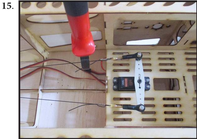
Cut off excess cable as shown.
