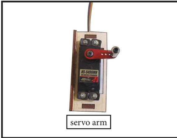
Install throttle servo into servo mounting tray
