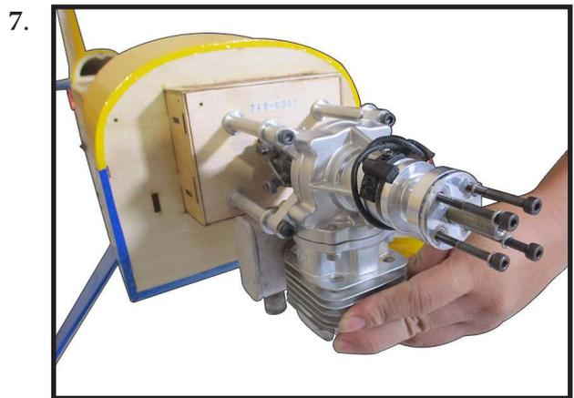
Use a 5.2mm bit to drill the engine mounting holes.
