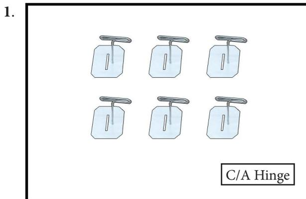
Remove each hinge from the wing panel and flap and place a T-pin in the center of each hinge. Slide each hinge into the aileron until the T-pin is snug against the aileron. This will help ensure an equal amount of hinge is on either side of the hinge line when the flap is mounted to the wing panel.
