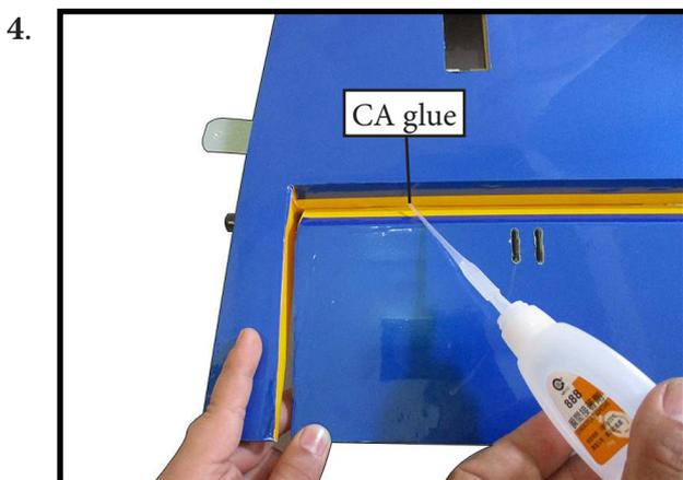
Turn the wing panel over and deflect the flap in the opposite direction from the opposite side. Apply thin C/A glue to each hinge, making sure that the C/A penetrates into both the flap and wing panel.
