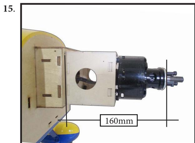
Then, use 5mm drill bit to enlarge the holes on the electric motor box.
