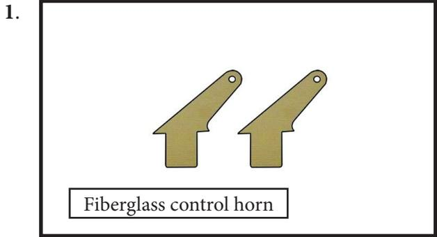
Use sandpaper to scuff the bottom of the aileron and flap control horns. Use a paper towel and isopropyl alcohol to remove any oils or debris from the control horns.
