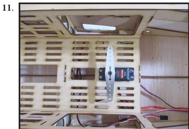
Feed one rudder cable through the pre installed cable exit tube in the rear of the fuse toward the front of the fuse. Repeat for other side.
