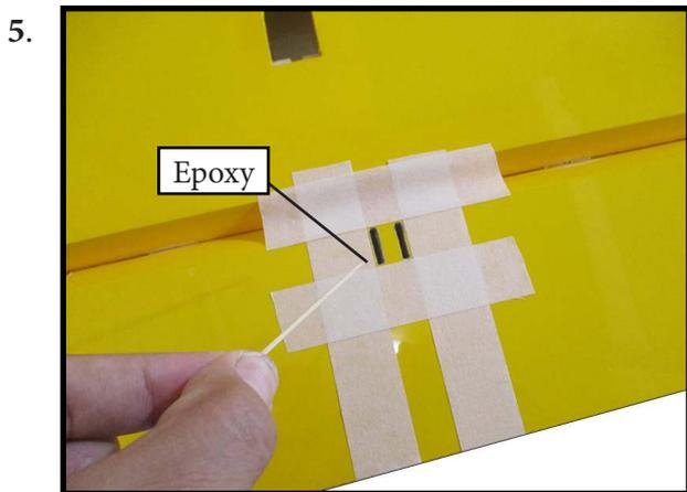
Apply epoxy to the area of the control horns that fit into the slots. Use enough epoxy so the control horns will be fully bonded to the fixed surfaces.
