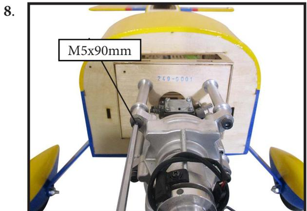
Tighten mounting bolts and secure engine to firewall.
