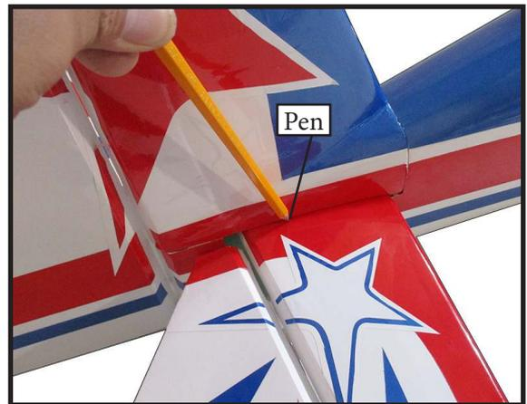
Remove the stabilizer. Using the lines you just drew as a guide, carefully remove the covering from between them using a modeling knife.
