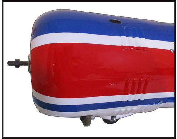
Install the muffler and muffler extension onto the engine and make the cutout in the cowl for muffler clearance. Connect the fuel and pressure lines to the carburetor, muffler and fuel filter valve. Secure the cowl to fuselage using the M3x10mm socket head screws. Putting a small length of silicon fuel tube under the head of the screw helps with vibration.
