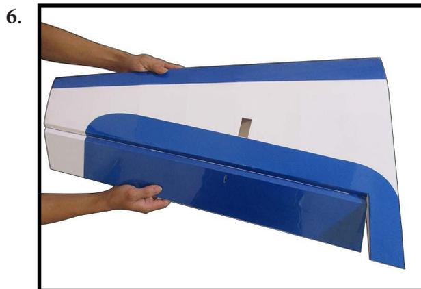
Turn the wing panel over and deflect the aileron in the opposite direction from the opposite side. Apply thin C/A glue to each hinge, making sure that the C/A penetrates into both the aileron and wing panel.
