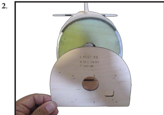
Locate the engine mounting in position on the firewall. Use a 2.5mm drill bit to drill the holes necessary to mount your particular engine choice.
