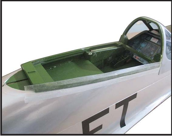
Use double-sided tape to temporarily stick it, then remove it and apply glue.
