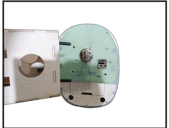
Attach the electric motor box to the firewall centered with the cross lines drawn on the electric motor box and firewall. Using M5x30mm to secure the motor box to the firewall. Please see pictures below.
