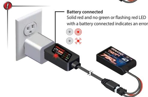
**Important! If the battery is damaged or defective, the charger's green LED will not come on and the red LED will glow solid or flash. Disconnect the battery. DO NOT attempt to charge the battery.**
