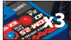
**Note:** If you missed the mode you wanted, keep the EZ-Set button pressed down and the blink cycle will repeat until the button is released and a mode is selected.
