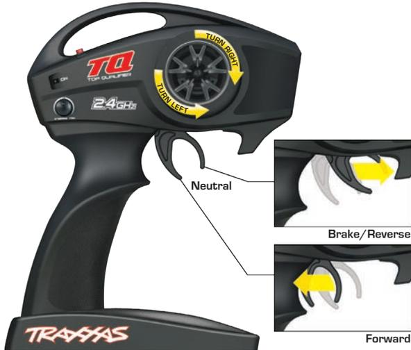
**i** For maximum radio range, hold the transmitter upright and pointed in the direction of the model.
