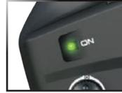
If the status LED flashes red, the transmitter batteries may be weak, discharged, or possibly installed incorrectly. Replace with new or freshly charged batteries. The status LED does not indicate the charge level of the battery pack installed in the model. Refer to the Troubleshooting section on page 16 for more information on the transmitter status LED codes.
