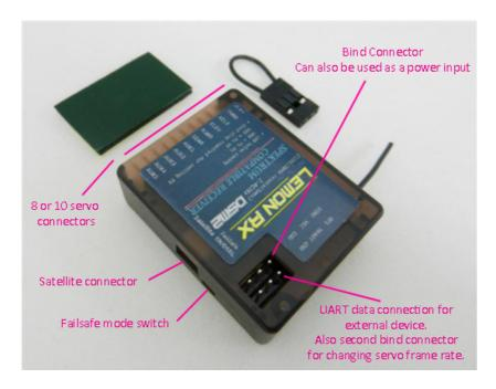
On these receivers there is a connector next to the bind connector labeled "UART". This is a serial connection, which can provide data to other external devices such a controller or on-screen display. It is not used for a stand-alone receiver. However a second bind plug can be used in this connector to enable an 11mS refresh rate for high-speed digital servos (see below).
