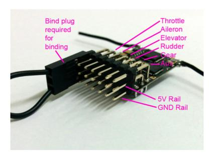
The 6 channel Ultra Light – with JST-ZH 1.5mm pitch connectors.
