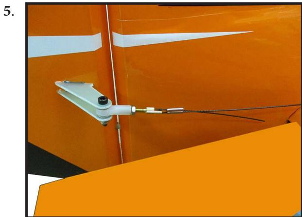
Loop the cable back through the brass swage tube and tighten the second loop through the brass swage tube as shown.
