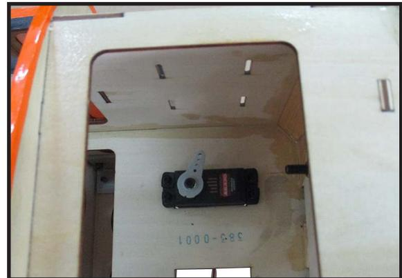
Reinstall the servo horn by sliding the connector over the pushrod wire. Center the throttle stick and trim and install the servo horn perpendicular to the servo center line.
