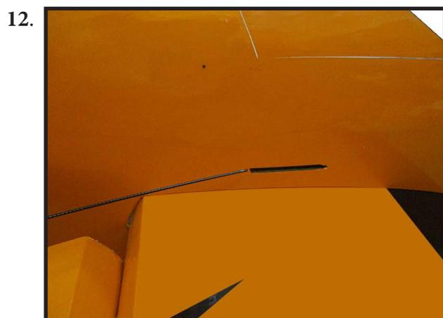
Thread cable through brass swage tube.
