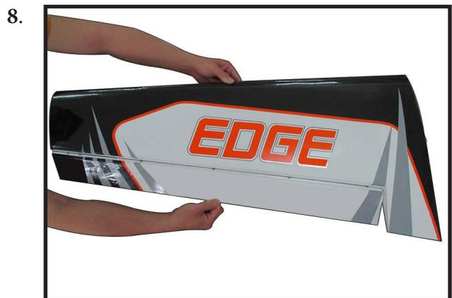
Check the fit of the aileron to the wing. The top of the ailerons will align to the top of the wing. Make sure movement is smooth and bind free.
