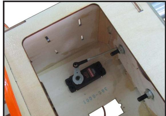
Move the throttle stick to the closed position and move the carburetor to closed. Use a 2.5mm hex wrench to tighten the screw that secures the throttle pushrod wire. Make sure to use threadlock on the screw so it does not vibrate loose.
