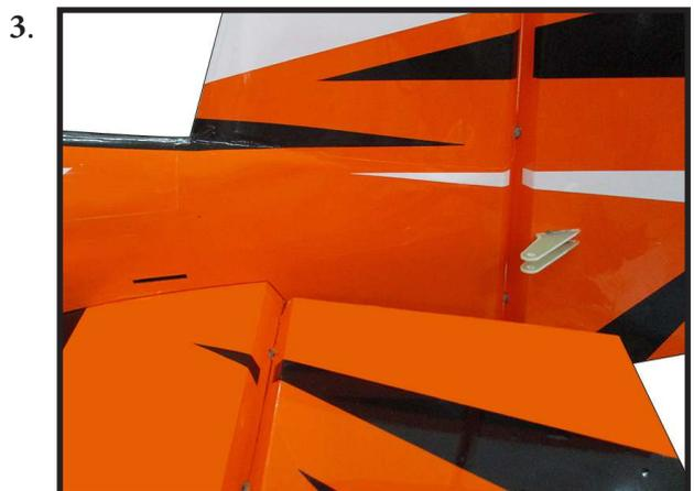
Thread the rudder cable through a brass swage tube, then the threaded coupler, and back through the brass swage tube on both sides. Pull light tension on the cable through the coupler on both sides as shown.
