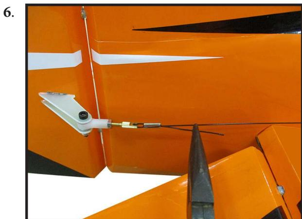
Crimp the brass tube with a crimping tool or pliers.
