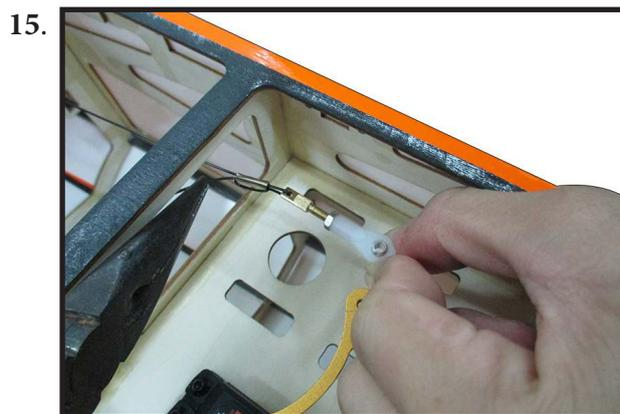
Crimp the brass swage tube with a crimping tool or pliers.
