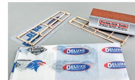
Lightly sand the airframe to get a neat, bump free finish before covering.
