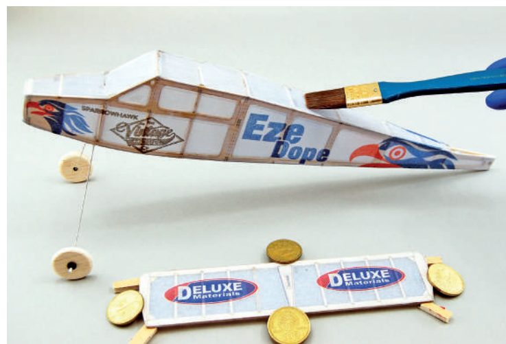
Painting on the Eze Dope mix with a very soft brush.
