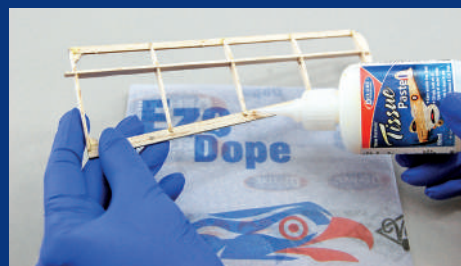
Whether wet or dry, you need to use Tissue Paste to apply your tissue. Squeeze a thin bead on the outer perimeter of each section.
