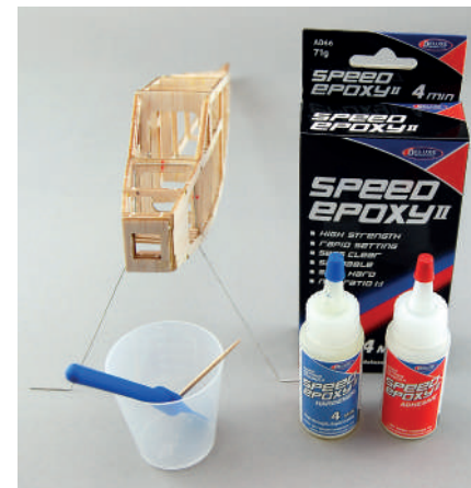
Speed Epoxy was used to stick the wire undercarriage to the Sparrowhawk.
