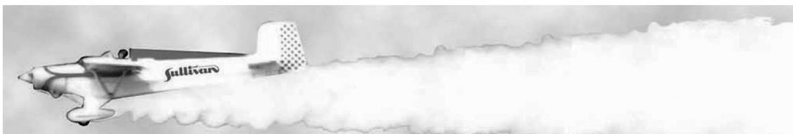
2) 50% Diesel & 50% Concrete Form Release Oil: Concrete Form Release Oil is obtained from the construction industry, industrial equipment and major petroleum companies such as Sunoco, Chevron, and Exxon. (Example: Texaco Canopus 13, Exxon Unuis 15, and Sunoco 22). They are available in five-gallon pails and drums. Diesel will make your smoke grayish, and harm the color of the covering on the fuselage bottom.
