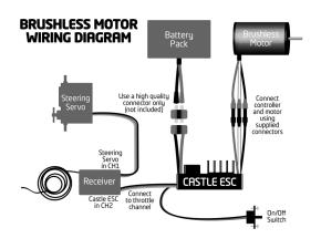
There is no polarity on the three ESC-to-motor wires, so do not worry about how you connect them initially. You may find it necessary to swap two wires if the motor runs in reverse. This will be explained below.
