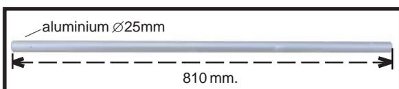
\*\*\* Test fit the aluminium tube dihedral brace into each wing haft. The brace should slide in easily. If not, use 220 grit sand around the edges and ends of the brace until it fits properly.
