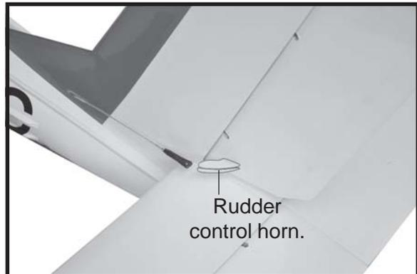
**RUDDER PUSHROD INSTALLATION.**
