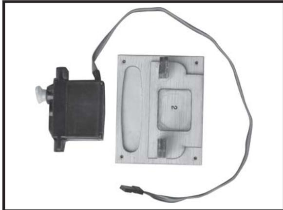
□ 3. Drill 1,5mm pilot holes through the block of wood for each of the four mounting screws provided with the servo. Install servo into aileron servo tray as same as picture below.
