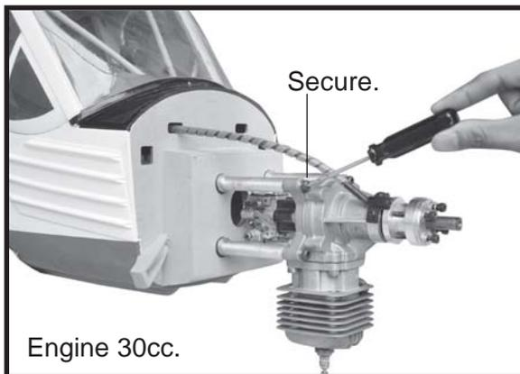
**INSTALLING THE THROTTLE - CABLE.**
