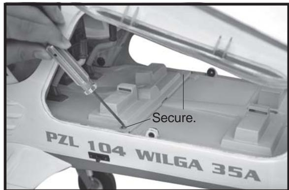
**INSTALLING THE COCKPIT.**
