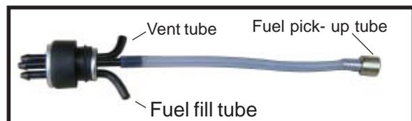
□ 6. When satisfied with the alignment of the stopper assembly tighten the 3mm x 20mm machine screw until the rubber stopper expands and seals the tank opening. Do not over tighten the assembly as this could cause the tank to split.
