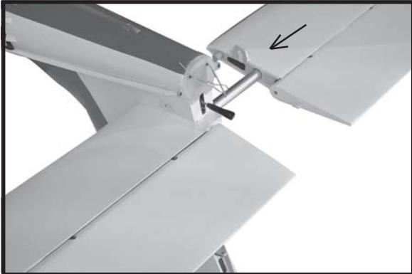
**ELEVATOR CONTROL HORN AND ELEVATOR PUSHROD INSTALLATION.**
