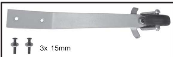
□ 2. Using a pen, mark the locations of the two mounting screws. Remove the tail wheel bracket and drill 1mm pilot holes at the locations marked.
